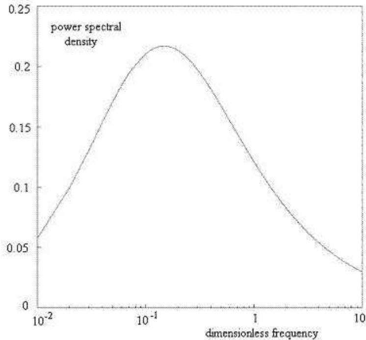
Fig.1. Dimensionless power spectra density function for wind velocity, after Eurocode 1 (BS EN 1991-1-4, 2005).
